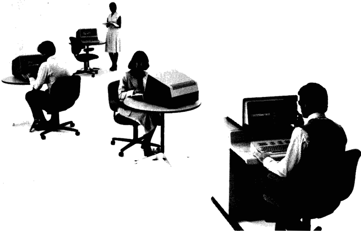
Hewlett-Packard 300 Computer System supports as many as 16 terminals.
