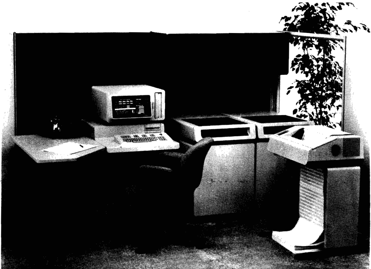
Hewlett-Packard 300 Computer System with optional HP 7925 125 Mbytes disc equipment and HP 2631 180 CPS serial printer.
